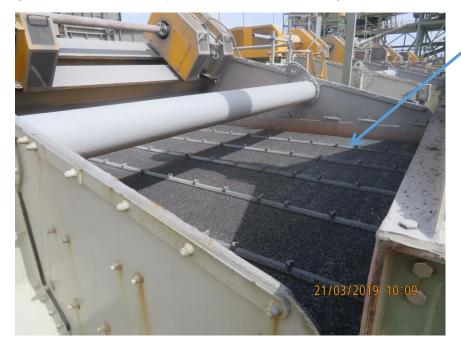
Blinding of a conventional vibrating screen
