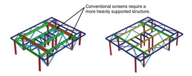
FIG 2 – Comparison between support structures for conventional screens and high frequency screens.
