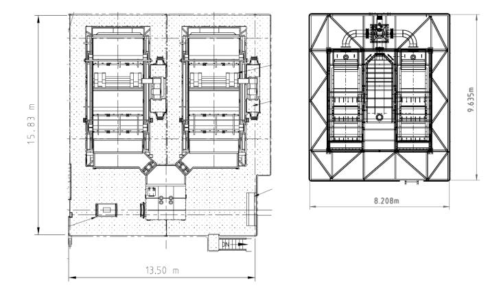
FIG 3 – Size comparison between conventional cyclone overflow trash screens - left (Lycopodium 2011) and HFLS - right.
